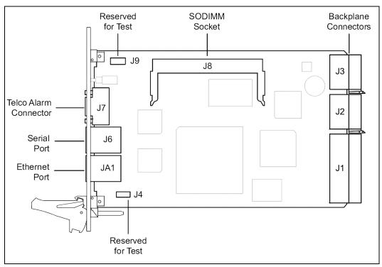
Figure 6. Backplane Connectors - Pin Locations
